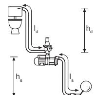
\*If  $H_s$  is 5m, a submersible pump should be used.
