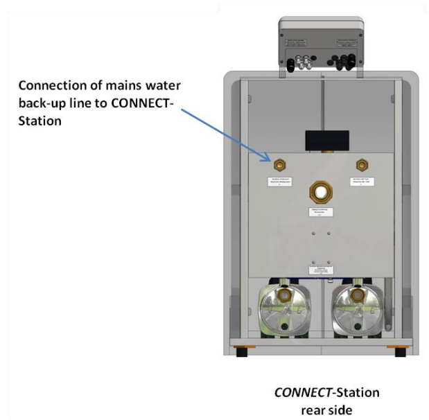
Figure 8: The mains water back-up is connected on the rear side of the CONNECT station
