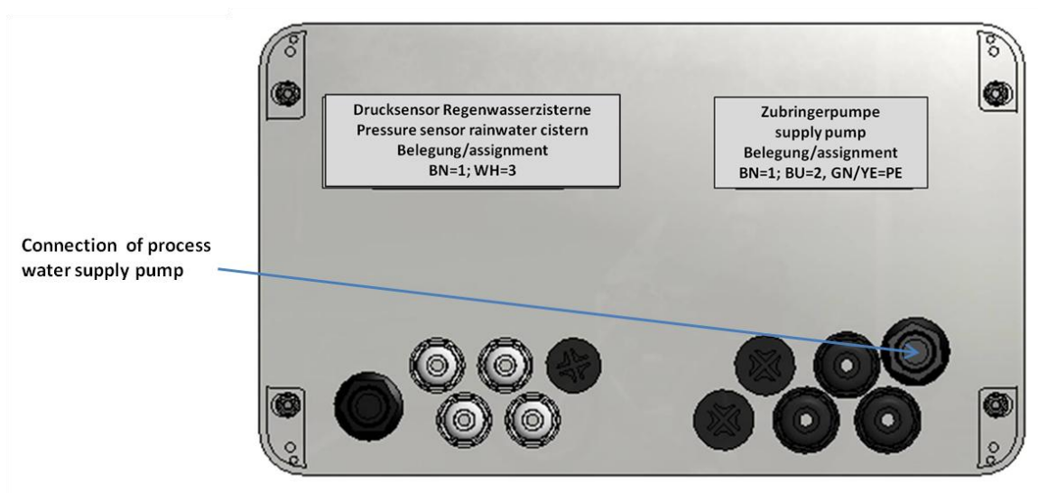
Figure 15: Connection of the process water supply pump to the CONNECT control unit
