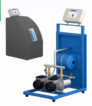
The double pumps are fitted to a metal frame with rubber buffers and the well-designed and sound-absorbing cover plate makes this system an asset for any plant room. DEHOUST**CONNECT** regulates the alternating start-up of the pumps and switches on the second pump when needed during peak extractions. Pressure sensors carry out the regulation, so that the switchpoints can be freely entered.
