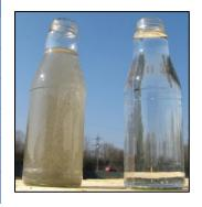
Effluent qualities on treated greywater comply with European standard EN 16941-2 and British Standard 8525-1 as well as European standard bathing water 2006/7/EG for safe water reuse.
