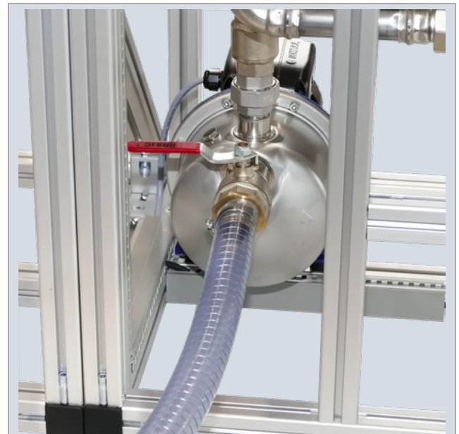
Figure 9: Attach the 1 ¼ inch (GWtec® 140/240) and 1 ½ inch (GWtec® 340/440/540/640) PVC hose to the filtrate pump using the (three-part) brass pipe union.
