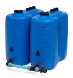
The lower connection pipe AQF, separately lockable with stopcock 1  $\frac{1}{2}$ ", is suitable for PE-storage containers AQF 570 to AQF 1500 liters blue or black. The connection pipe has been developed for the on-site connection of the DN50 PE pipe or D=63mm hose.
