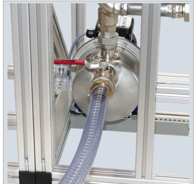
Figure 9: Attach the 1 1/4 inch (GWtec® 140/240) and 1 1/2 inch (GWtec® 340/440/540/640) PVC hose to the filtrate pump using the (three-part) brass pipe union.
