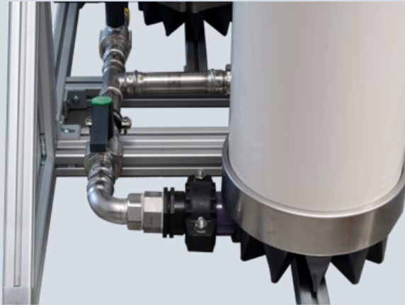
Figure 6: Bottom connections shut-off 2
